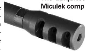
You can make effective changes without removing material through "Clocking". This is simply indexing where the comp is positioned at final assembly. Many a right shoulder shooter will report an "up and to the right" movement in recoil. To combat that, "clock" the comp (very near the 1:30 position) to vent its upward gas flow in the same direction.
