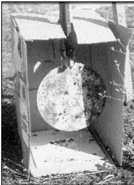
**Simple but effective.** Pat Kelley wrapped a cardboard box around a steel flash target to test fragmentation characteristics of the different slugs.
