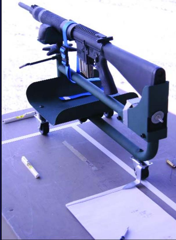
**"The Sled" consisted of a Caldwell rifle rest on rollers. Smooth rollers gave repeatable results with even the modest recoil of a compensated .223.**
