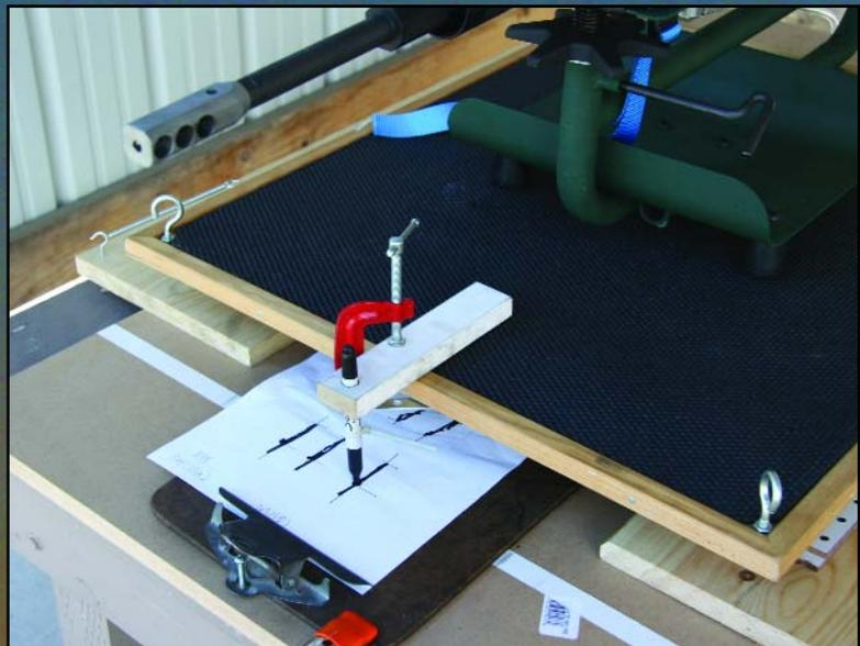
Roller Ball 2 in action. Kelley's rest rode on a bed of material-handling ball bearings, allowing the rest to slide easily both front-to-back and left-to-right. Note the recoil-tracking Sharpie™ in the foreground.
