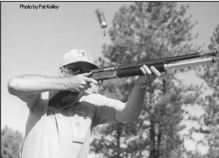
**Long recoil Auto-5's shoot faster than you think. Pat Kelley's race-5 appears barrel-forward (above) and barrel-back (in recoil, below). Note the position of the muzzle relative to the end of the mag tube.**
